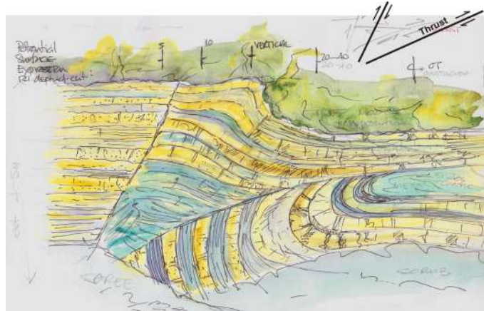
Figure 5 Illustration of a fault – thrust duplex typical of those seen in this area. This example is taken from the field notebook for Wax Hall (SO 297 759).
