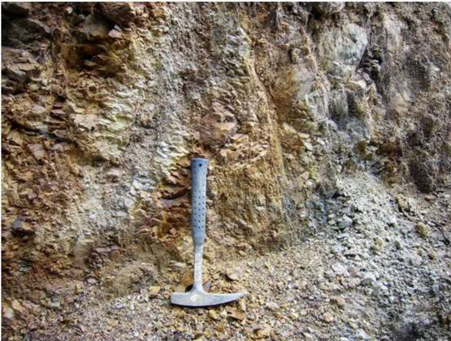
Plate 2.7. Tectonised quartz arenite (Martley Quartzite) in Martley Rock Fault Zone in north wall of the side trench. Hammer is 32 cm long. (William Barclay)
