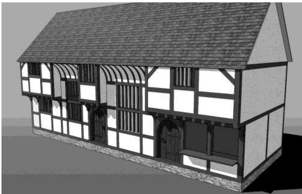
Figure 11. Tudor Cottage, Broad Street, Weobley. Reconstruction of the two half-Wealden houses hidden within the present fabric - that on the right forming a shop with adjacent hall
