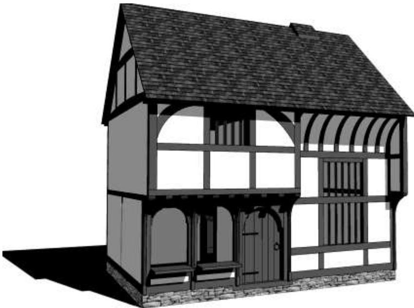
Figure 18. No. 4 Portland Street, Weobley. A reconstruction of this half-Wealden house, one of three similar units, illustrating the shop with jettied solar above and an open hall to the side
