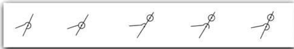
Figure 7. The Old Priory, Titley. Assembly marks, 1 to 5 by quarter circle increments
